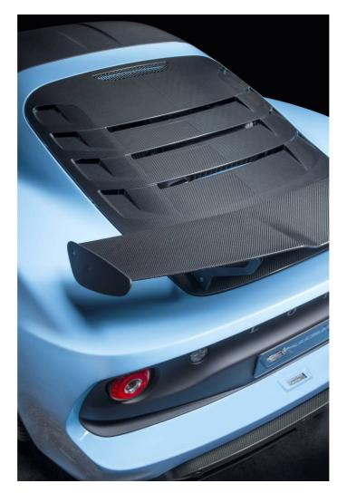
Distinctive in its appearance, thanks to wider aperture grilles in the new front clam panel, the Exige Sport 410's revised aero configuration provides total downforce of 150 kg (60 kg at the front and 90 kg at the rear); developed through extensive CFD modelling and wind tunnel testing in order to preserve the car's handling balance and high-speed stability.
